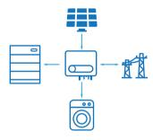
During daylight hours with sufficient sunlight (clear weather), solar photovoltaic (PV) generation first charges the battery up to its maximum charging capacity. Any surplus electricity after achieving maximum charge is then used to supply household loads. If the PV system cannot meet the full electricity demand of the loads, electricity is supplemented by purchasing from the grid.
