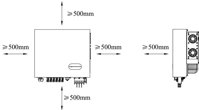
When installing multiple inverters, a certain spacing should be reserved between the inverters. The recommended installation method is the herringbone shape as follows.
