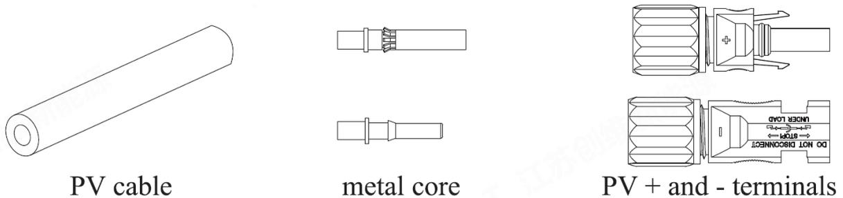
Step 2: Strip the wire with a wire stripper to  $7 \pm 0.5mm$  as shown in the following figure.
