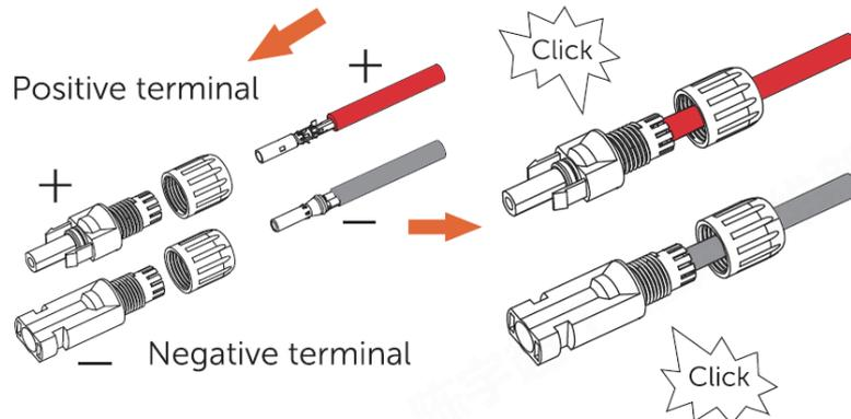
Step 6: Tighten the nut and use a multimeter to measure the photovoltaic voltage of the DC input to verify the polarity of the DC input cable.
