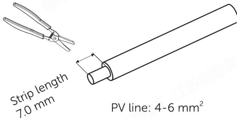
Step 3: Tighten the cable with the insulation layer stripped and insert it into the metal core (see Figure 1), and ensure that all wires are inserted into the metal core (see Figure 2).
