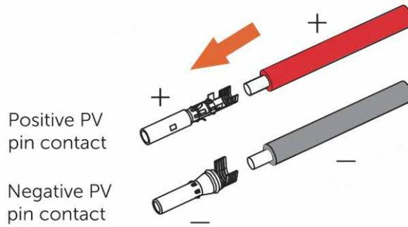
Step 4: Use a crimping pliers to compress the cable wire and the PV terminal metal core tightly to ensure a firm crimping connection.
