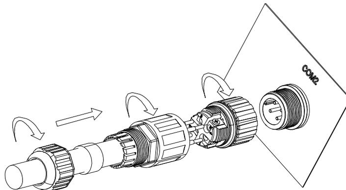
Step 3: Insert this terminal into the COM2 port of the inverter and rotate it clockwise to lock.
