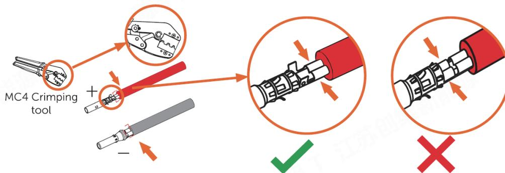
Step 5: Pass the crimped positive and negative cable wires through the locking nut and insert them into the corresponding plastic shells respectively until a click sound is heard, indicating that the metal core has been snapped into place.
