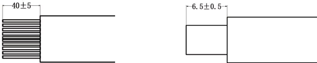
Step 2: Terminal the core wire/immerse it in tin to ensure that the copper wire is not dispersed.
