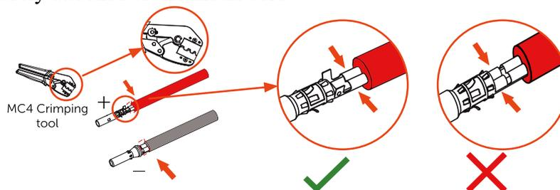
Step 5: Pass the crimped positive and negative cables through the locking nuts and insert them into their respective plastic housings until you hear a 'click' sound, indicating that the metal cores are securely locked into place.
