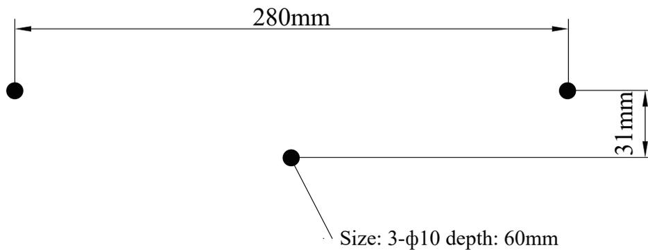
Step 3: Use a hammer to slowly knock the expansion tube into the drilled hole, and fix the bracket with the expansion screws in the accessory bag of the inverter.
