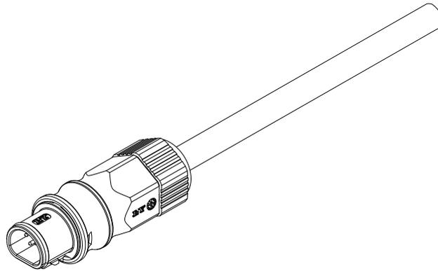
Step 6: Align the COM port slot at the bottom of the inverter and insert this terminal.
