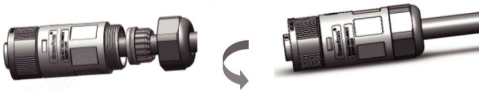
Step 4: Mating plug and socket: Push the locker onto the socket housing completely, then rotate the locker according to the direction instructed by the marks on the locker. (Warning: hold the body)
