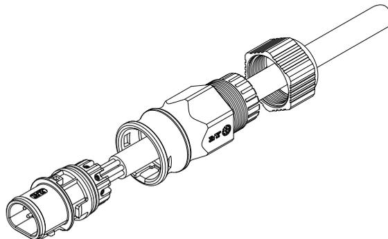
Step 4: Push the main component into the rubber core and assemble it into place when you hear a clicking sound.
