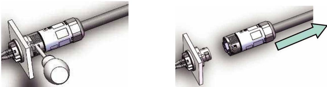
Step 2: Disassembling body and housing for rewire.
