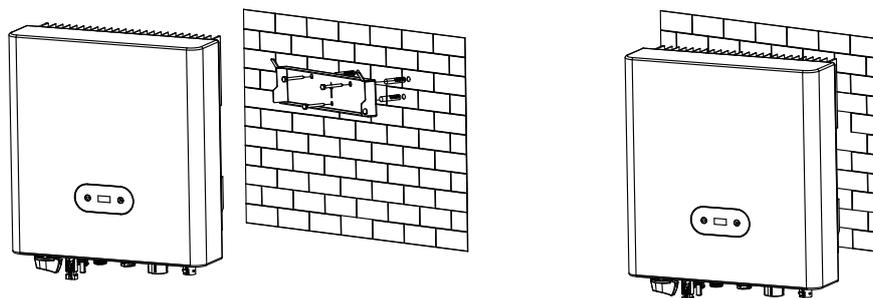
Step 3: After confirming the inverter is fixed reliably, Using M5 Phillips screw in accessory bag to lock the inverter to the bracket.
