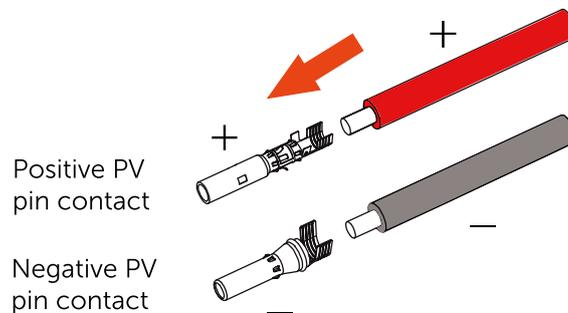
Step 4: Use a MC4 terminal crimping tool to firmly crimp the cable with the PV metal core, ensuring that the cable is securely attached to the metal core.
