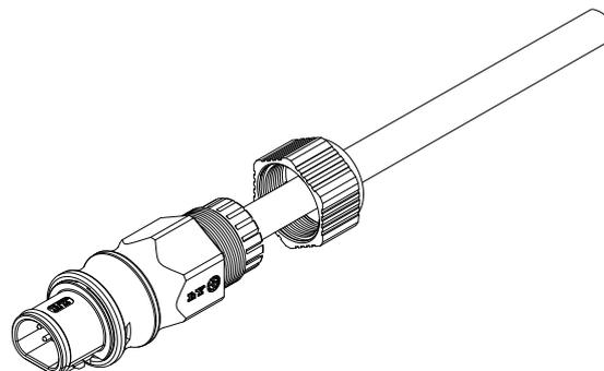
Step 5: Tighten the nut to the main body. (Suggested tightening torque of  $3.5 \pm 0.5$  N.m).
