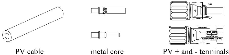
Step 2: Use the wire stripper to strip the wires to a length of  $7 \pm 0.5$  mm, as shown in the diagram below.
