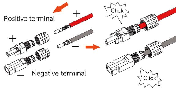
Step 6: Tighten the nuts and use a multimeter to measure the DC input PV voltage to verify the polarity of the DC input cables.
