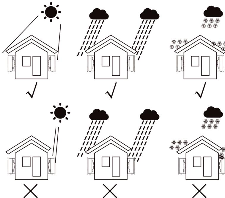
Install the inverter at a maximum back tilt of 15 degrees, the inverter can not be tilted forward, inverted, excessive back tilted or side tilted.
