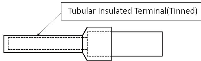
Step 3: Insert the cable into the main component and lock the screw with a Phillips screwdriver. (Recommended tightening torque for screws is 0.1~0.2N. m)
