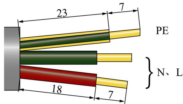
Step 2: Fix the wires into the correct position. Torque 0.8N.m Please try to pull out the wire to make sure the it's well connected.
