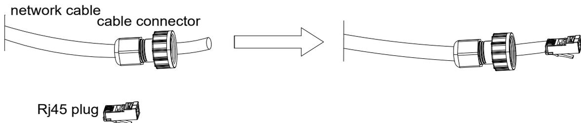
Step 3: Insert the cable connector into BMS port at the bottom of inverter and screw it tightly.
